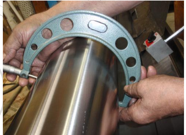
These work rolls, for a coil converter, have been precision ground and are ready to return to service as part of a flattening operation.
