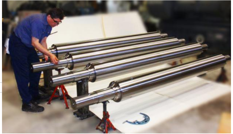
These work rolls, for a coil converter, have been precision ground and are ready to return to service as part of a flattening operation.
