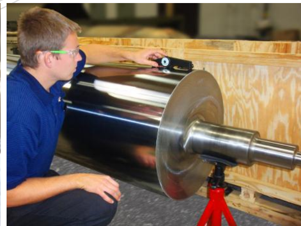
Here a Menges Engineer inspects a recently chrome plated heat transfer roll. Using a special tool, he is measuring the thickness of the mirror-finish chrome.
