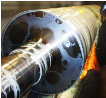
The above roll is being cylindrically ground and will be re-plated in chrome.
