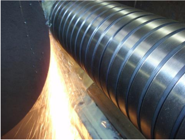
This serrated roll needed a very exact diameter & low TIR. Here we see it at the preliminary grinding stage.
