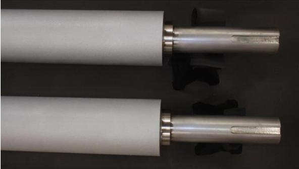
*These twin rollers have been acid etched, creating a matte finish along the roller face. This finish adds a certain amount of friction as the roll meets the web.*
