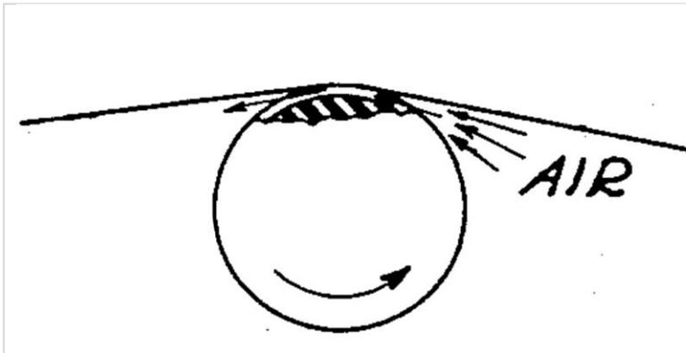
*Every plant manager should realize that loss of friction between the roller and web can potentially lead to wrinkling. One of the leading causes of loss of friction is air entrapment between the web and roll. This can be caused by a number of factors.*
