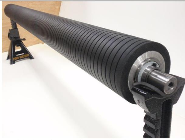
*Wedshaft web spreader completely assembled.*
